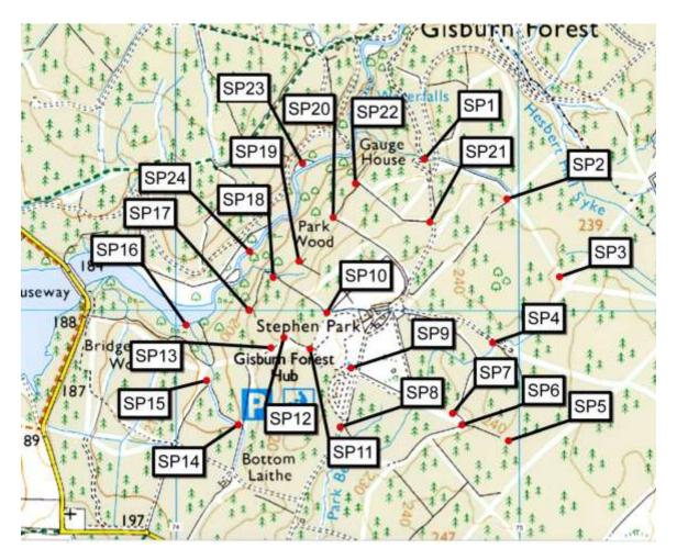
Figure 17: Survey nodes transposed from the tithe and first-edition 6-inches to 1-mile maps onto modern 1:25,000 OS mapping. This figure contains OS data © Crown copyright and database rights (2016).
