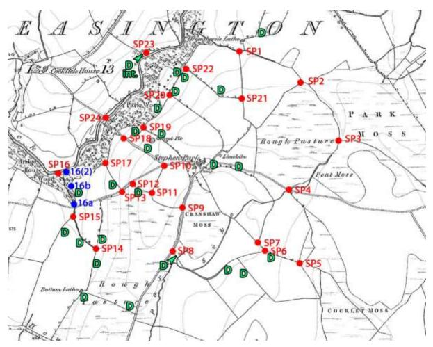
Figure 33: Location of ditches with respect to the banks on the boundaries shown on the 6-inches to 1mile (1:10,560) OS map surveyed in 1847. Banks without ditches are not marked. 'D' touching a mapped boundary shows the ditch location with respect to the bank marked by the line. The boundary between SP2 and SP5, via SP3 and SP4, is not evident in the mossy conditions and dense forestry.
